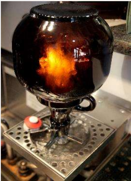
Water is blocked by the growler neck
