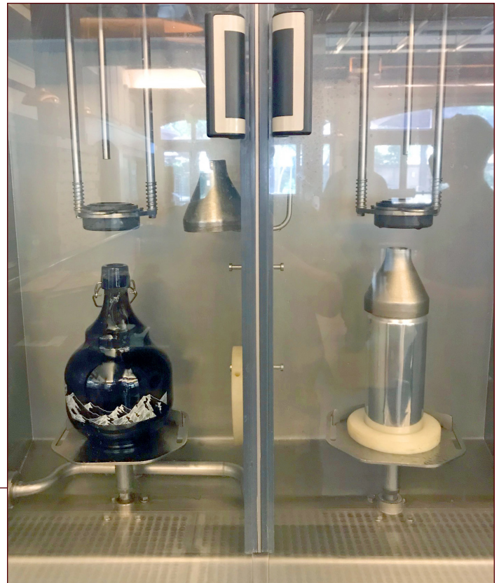
A growler filler can be adapted to fill draught to-go cans.
