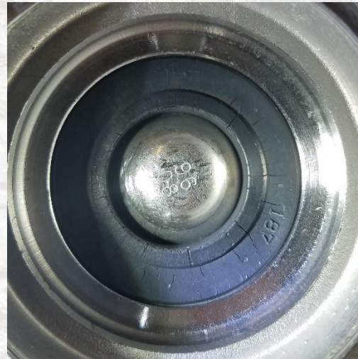
Cracked rubber from UV exposure (sunlight)
