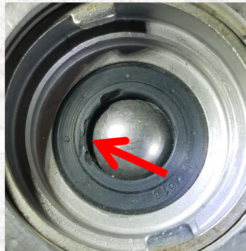
Impact damage to raised rim on CO 2 Valve
