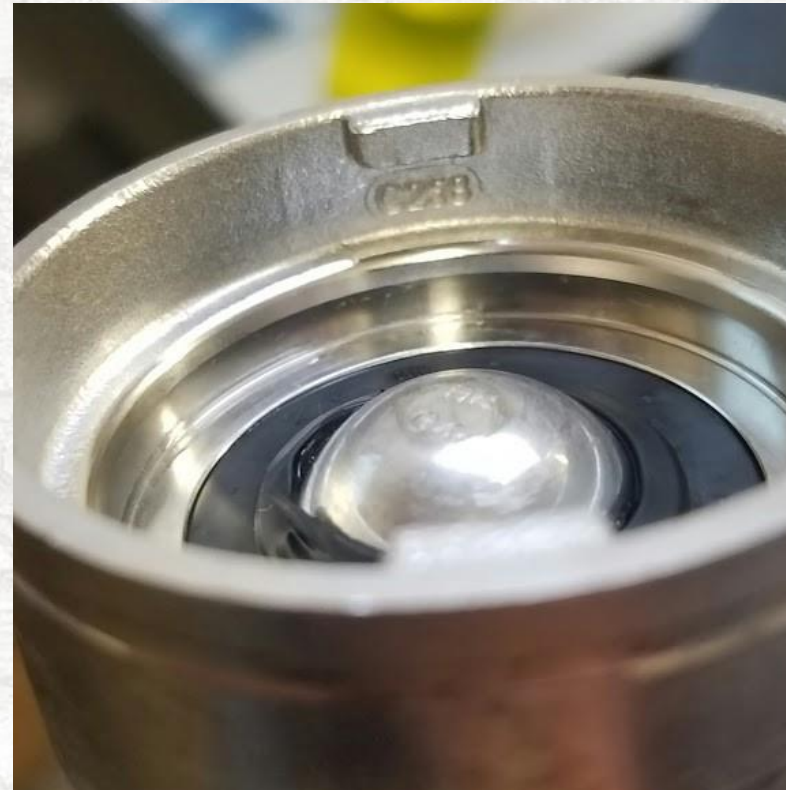
Poppet pushing through CO 2 valve
